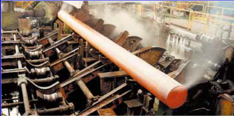
Pipe coming out of the expander
